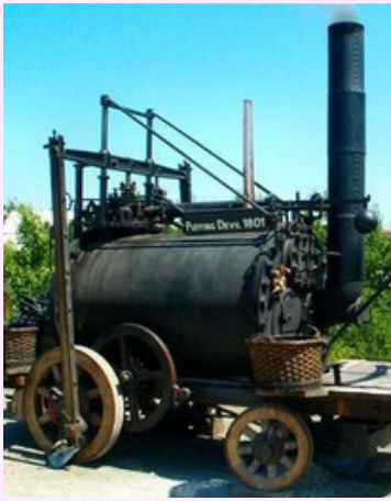
Replica of Richard Trevithick's 1801 steam road locomotive at the Royal Cornwall Show.
