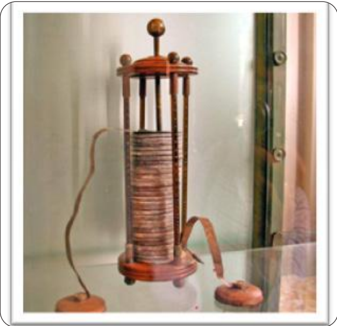
(The voltaic pile was made of alternating copper and zinc conductive discs with a weakly acidic layer.)
