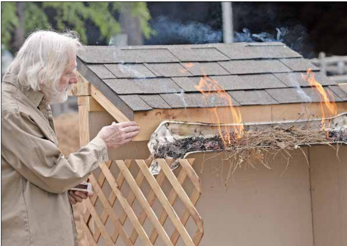
Steve Quarles demonstrates how embers can ignite dry leaf debris and melt plastic gutters.
