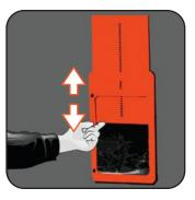
Step 3. Before placing the drive unit back, test the door if it runs smoothly. Adjust screws holding the frame if required.
