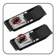
Step 2. Remove the square battery guard. Replace 2x AA alkaline batteries and place back the square quard.
