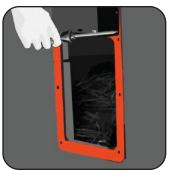
Step 1. Remove the drive unit by unscrewing 4 screws in the corners of black housing.
