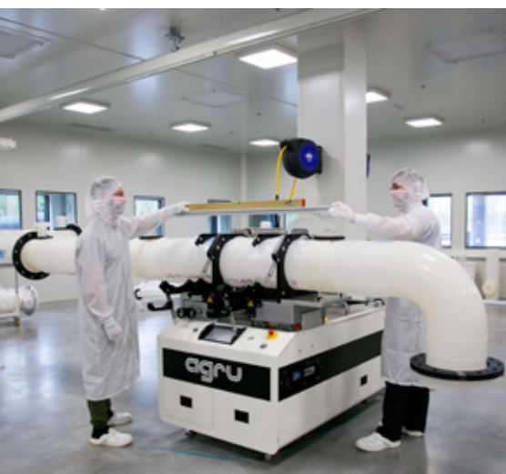
For high-purity applications, ready-to-use pipe isometries are produced in specialised fabrication shops around the globe
