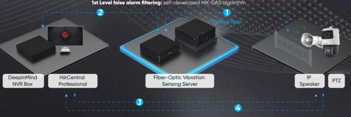
2st Level false alarm filtering: link with deep learning CCTV system
