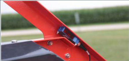
BaleEye sensor accurately detects bales on platform with no mechanical moving parts
