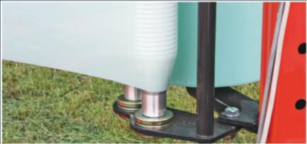
Proven pre-stretchers with 70% plastic stretch result in less plastic use
