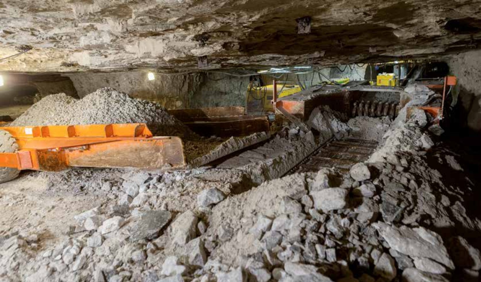
Joy battery hauler feeding Joy feeder breaker.
