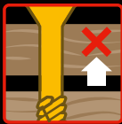
Partially Threaded Stops The Timber Jacking
