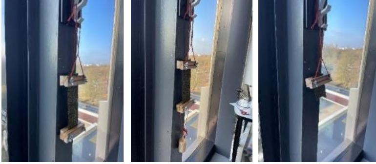
Figure D: From left to right; The basic set up for each sample strip with the two bases. The set up with one weight attached to the strip. If the weight became too much the strip would tear as seen in the last photo.
