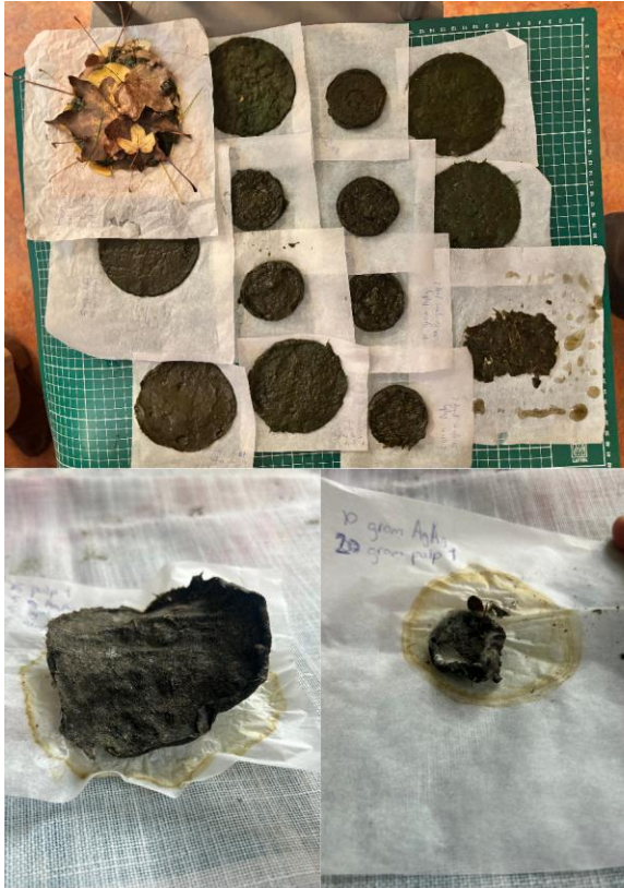
Thicker plateaus of materials which started molding in the end
