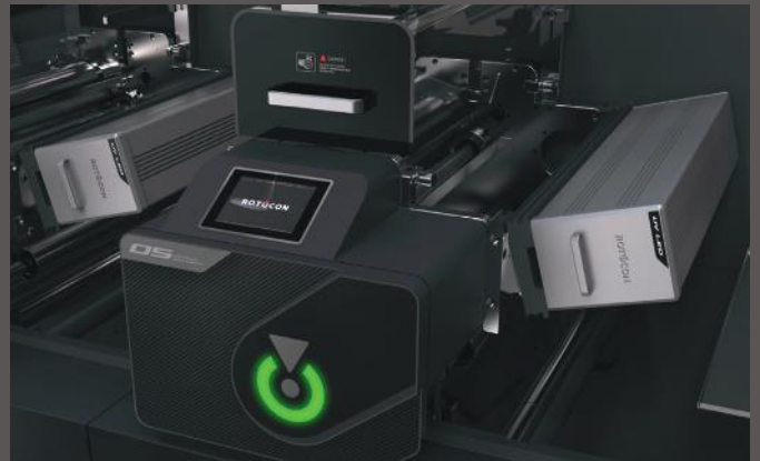
Sleeve system with three servos
