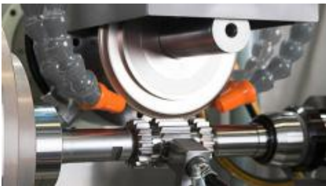
Fig. 5: Machining of a triple pinion © KAPP NILES
