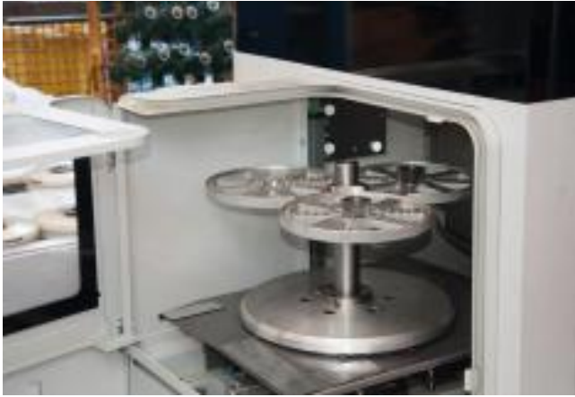
Fig. 3: The multifunctional axis allows the extraction of measuring and test parts © Martin Witzsch
