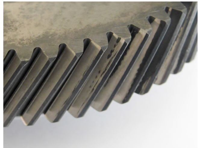
Fig. 9: Tooth flanks of a continuously generative-ground gear that has not been smoothly ground in certain areas
