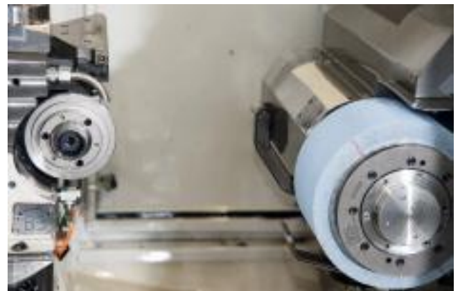
Fig. 5: The diamond dressing roll on the left in the picture can be used on all machines © Martin Witzsch
