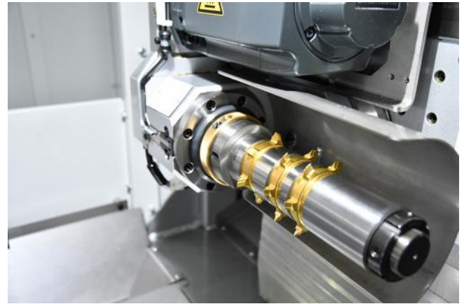
Fig 7: Assembly to perform the new ChamferCut process in a dedicated ChamferCut unit
