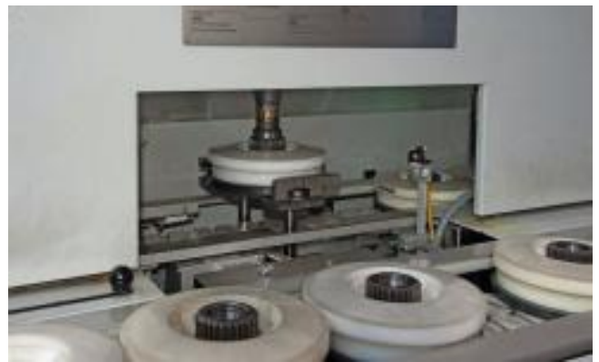
Fig. 2: The pick-up unit removes a finished workpiece and loads a blank part on the workpiece spindle © Martin Witzsch
