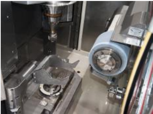
Fig. 4: Here, the interchangeable prism (left below) swivels out of the park position and ready to receive the screw © Martin Witzsch
