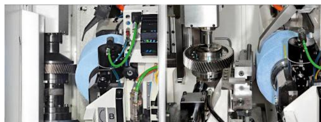
Image 1: A generating grinding worm during the grinding process (left) and while it is dressed (right).
