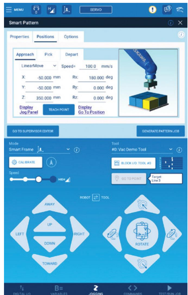
Smart Pattern from Yaskawa enables the quick development of jobs for repetitive handling tasks
