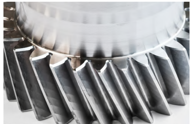
Fig 8: Examples for gears which are manufactured with the new ChamferCut process
