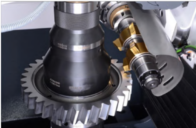
Fig 3: ChamferCut tool system for chamfering on a standalone machine
