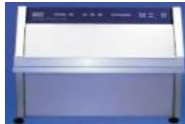
ACCELERATED WEATHEROMETER (QUV) ASTM G 154, ISO 16474
