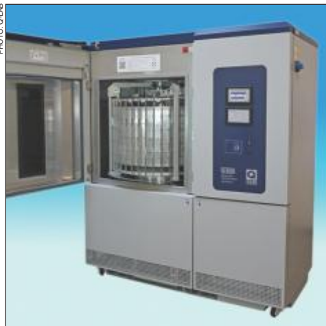
The Q-SUN Xenon Test Chamber uses a full-spectrum xenon arc lamp to reproduce the effects of full sunlight, including UV, visible light, and infrared radiation.
