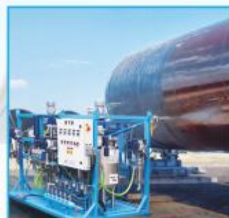
External Automatic Pipe Coating
