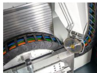
Image 3: The directly driven dressing spindle swivels between a working position and a parking position.
