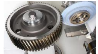
Image 2: The KNG 5P expert can be used to grind workpieces with a gear width of up to 670 mm.
