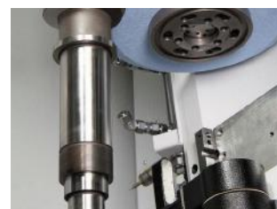
Image 5: The KNG 5P expert can be used to grind worms with pitch angles of up to 45 degrees.
