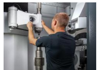
Image 4: The tailstock can be swiveled away and is infinitely adjustable to a tip pressure of up to 2,000 N.
