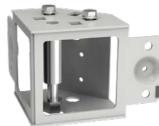
Plinth corner equipped with levelling bolt for SZB IT or DSR IT cabinet In order to fasten the levelling bolt in the corner and join the corner with the cabinet, 2 pcs. of M8 bolts with washers are used (delivered with the plinth corner).
