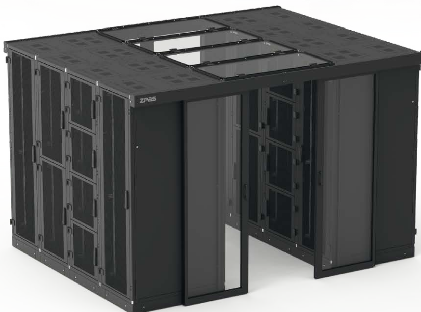
Example of Data Box set consists of: 4 pcs of SZB IT 42 U, 800 x 1000 mm, 2 pcs of DSR IT 42 U, 800 x 1000 mm with 2 compartments, 2 pcs of DSR IT 42 U, 800 x 1000 mm with 4 compartments, sliding doors, flat aisle roof. Cabinets on 100 mm plinth.
