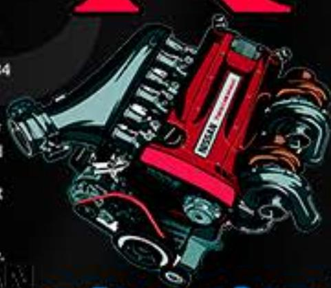
The last "Godzilla" of the 20th century featured upgraded ball-bearing turbos, providing phenomenal throttle response in an age where most boosted cars struggled with turbo-lag. The GT-R had a maximum theoretical output of 276 horsepower with the Japanese Gentlemen Agreement. But several independent tests have often claimed that the figure was somewhere north of 320 horsepower instead. With forged pistons and a cast iron block the tuning potential for the RB26DETT is phenomenal.
