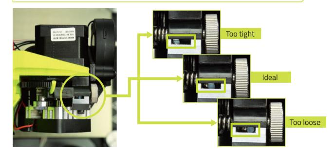
Solution Loosen the idler as needed by turning the silver idler adjustment knob clockwise. Squeeze in on the idler and insert filament into the feed hole and all the way through the idler until it is held in place by the extruder hobb. Once the filament is in place, retighten the idler to the tension shown below with about 2 millimeters on either side of the nut as seen through the window.
