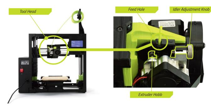
During printing, the idler holds filament against the extruder hobb which pushes filament down into the hot end. Correct idler tension is important for keeping filament flowing properly during the printing process. The idler tension can be seen by looking at the tool head from above. Rotating the idler adjustment knob clockwise will loosen the idler, while rotating counterclockwise will tighten the idler.
