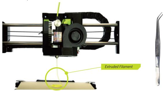
**9C** Wait ten seconds for the filament to cool, then remove the extruded filament with the included tweezers.
