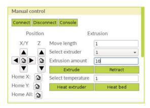
**9B** If you do not see filament coming through the nozzle and the drive gear stops moving, click the **Extrude** button once more and wait. Repeat as needed until you see consistent and repeatable extrusion.
