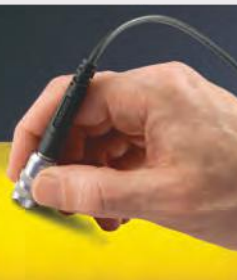
Duplex Probe measures individual layer thicknesses of zinc and paint in a duplex coating system
