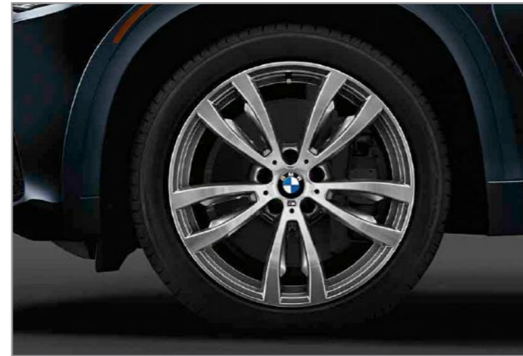
Double Spoke light alloy wheels (Style 469M) 20 x 10.0 front, 20 x 11.0 rear; and 275/40 front, 315/35 rear run-flat performance tires 1,2,3
