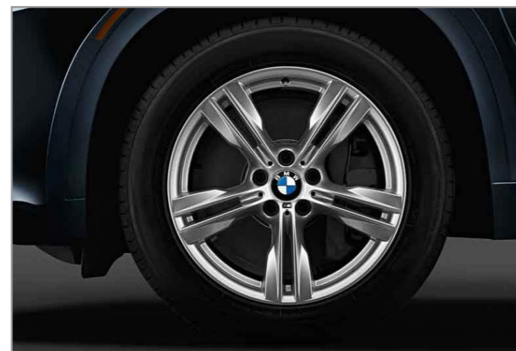
Double Spoke light alloy wheels (Style 467M) 19 x 9.0 front and rear; and 255/50 front and rear run-flat all-season tires 1,2
