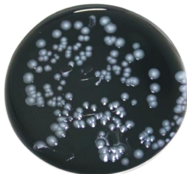
Figure 2: Legionella detected via the standard culture-based method (AS 5132:2017). The opalescent circles are the Legionella colony with each colony representing a colony forming unit (CFU).
