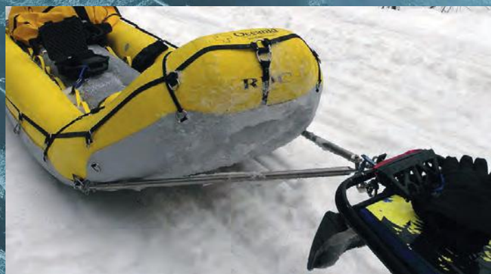
The Snowmobile Tow Package includes all necessary hardware and fittings, including protective tow shield and fittings, t
