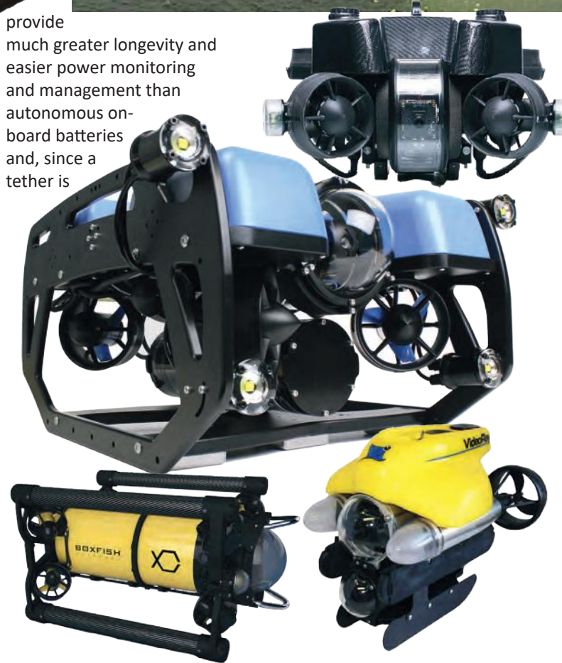
Pictures above: Top-right to bottom left- Deeptrekker's Photon , Blue Robotics' Blue ROV , VideoRay's Pro4 and Boxfish's ROV+
