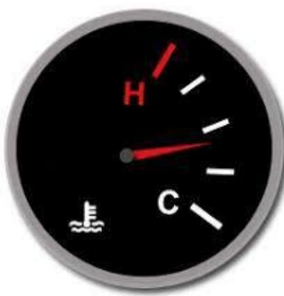
A Typical engine temperature gauge
