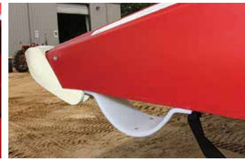
Inside & Outside Snouts with cutout for Height Control Sensor for Case IH 2200/2400/3200/3400
