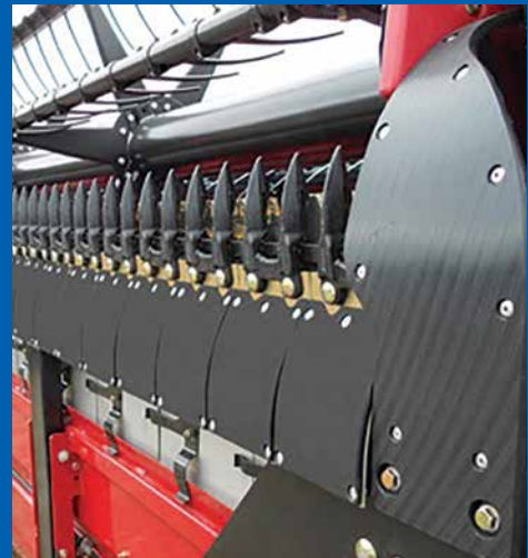
Predrilled & Counterbored Holes Protect Hardware. All Hardware is Included with Skid Shoes.
