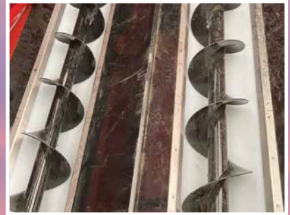
AUGER TROUGH & TUBE LINERS
