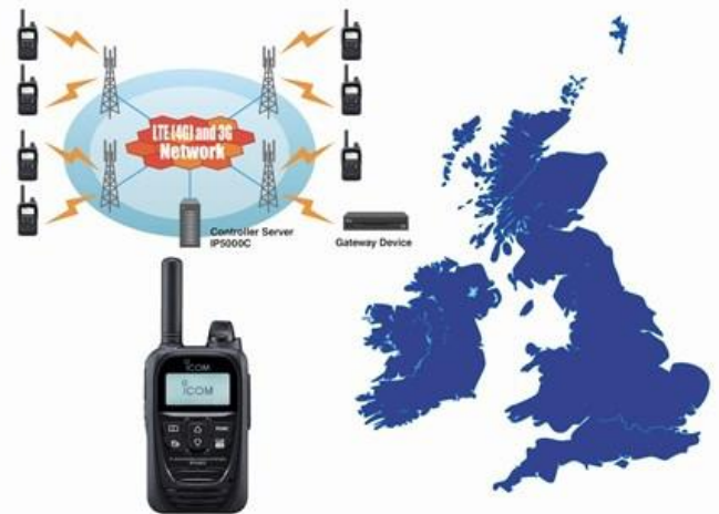
A typical POC radio system network
