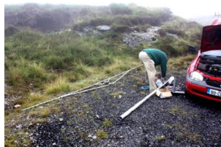
John EI7FAB assembling 23cm 55 element Tonna Yagi
