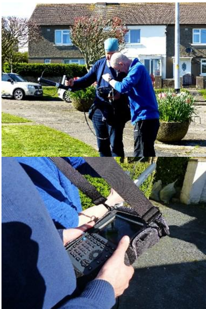
Fig. 5 Sweeping the area for a peak in the interfering signal
