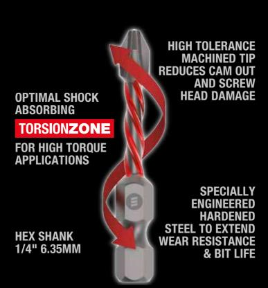
The specially designed "Torsion Zone" is created by combining the extra hardened steel with a softer central zone that allows a slight flex in controlled areas. This flex absorbs the peak torque created by power tools and prevents premature wear of the bit.
