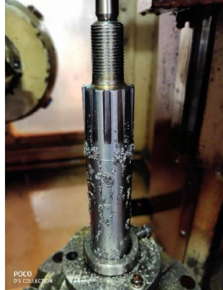
Setup on a Cooper P 254 hobbing machine
