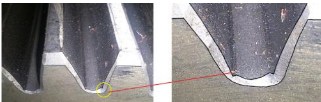
Fig 8: Notch found after gear grinding due to improper tool usage in gear cutting
