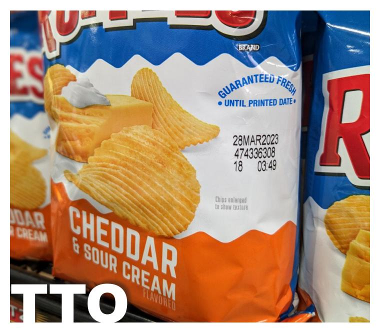
Near Edge thermal transfer printing operates at the speed of a packaging line. Thermal transfer overprint (TTO) ribbons print variable information directly onto the material, a method widely used in the food and beverage, medical and healthcare, and pharmaceutical industries, contributing to their efficiency and productivity.
