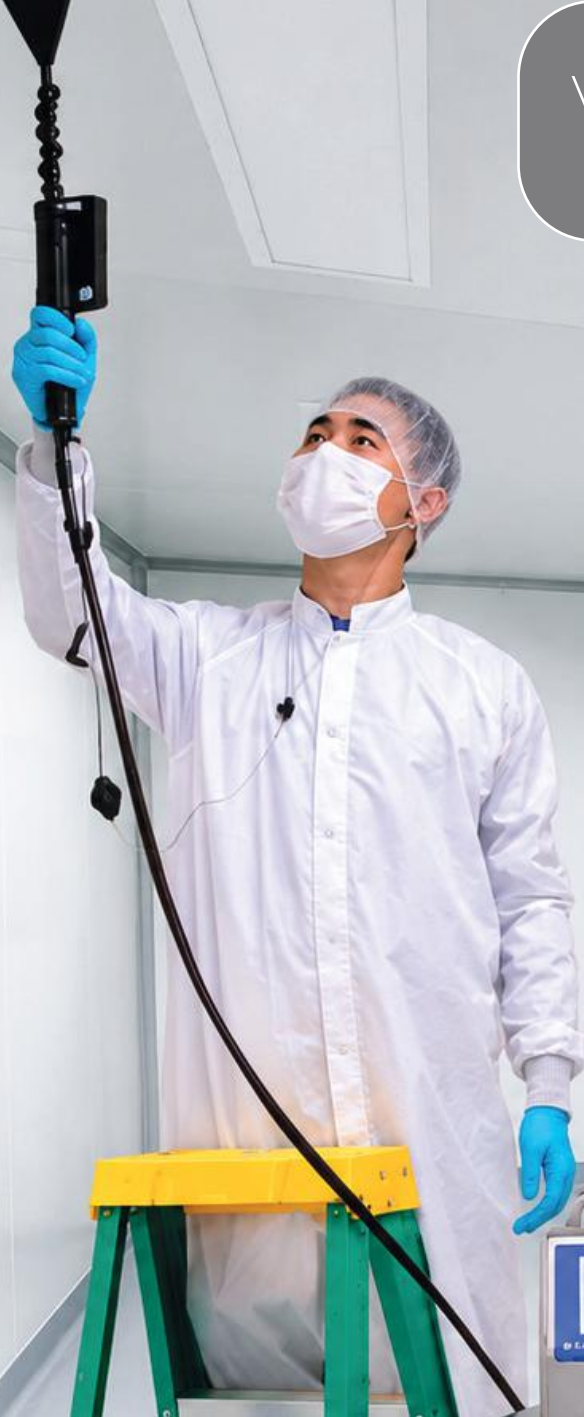
Fig.1 Cleanroom Certifier technician using filter integrity testing equipment following ISO 14644-3 standard.
