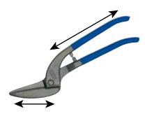
In standard tin snips, edges and handle are traditionally forged into one unit. The force required for cutting is determined by the ratio of edge length to the handle length.
