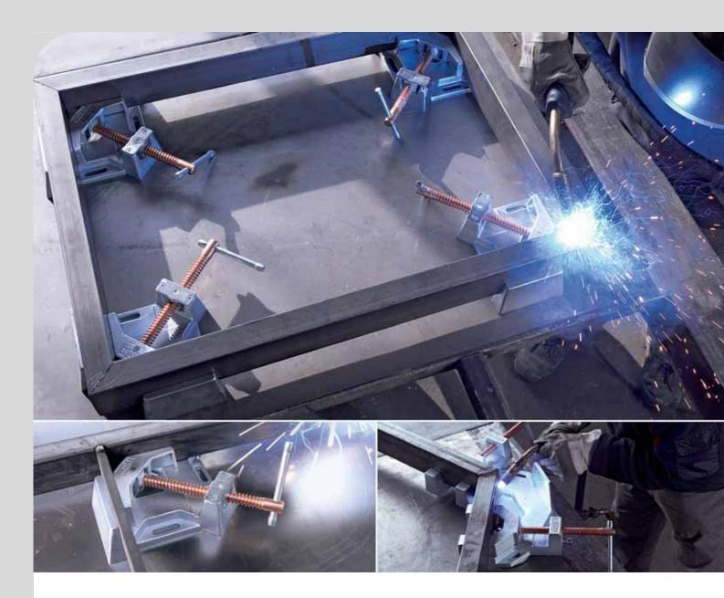
Unhindered access to workpiece during welding and assembly work
