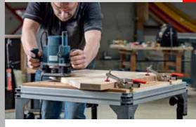
■ For using the BESSEY toggle clamps on multifunction tables such as Festool MFT and Sortimo WorkMo with hole diameter of 20 mm and plate thickness of min. 19 mm to max. 25 mm
