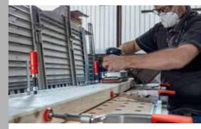
■ For using on multifunction tables such as Festool MFT and Sortimo WorkMo with hole diameter of 20 mm and plate thickness of min. 19 mm to max. 25 mm
