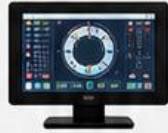
CNC CONTROLLER (STORE & SAVE CRIMPING COMBINATIONS)
