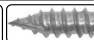
The Type 17 point will clean the existing hole of metal burrs & the oversized threads will generate increased holding strength.
