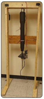
Figure 1: Prototype of the soil sampler
