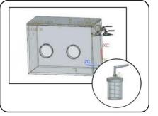
CAD Design of Sealable Box and Mixing Bowl
