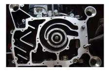
onstruction with monobloc base-cylinder and cylinder liners in anti-seize spheroidal cast iron brought back in wet.
