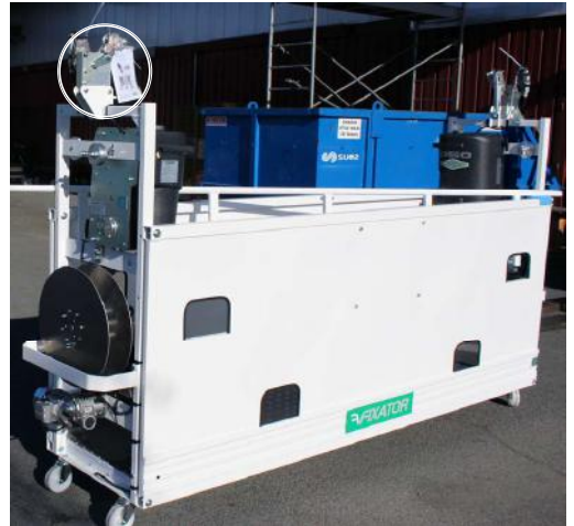
✓ FALL-PREVENTION DEVICE positioned on a stirrup
