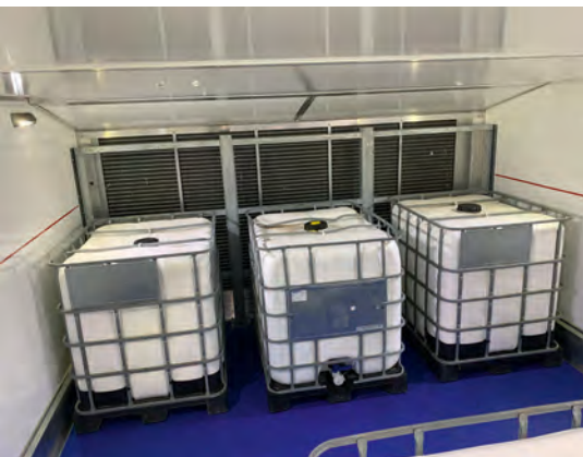
During the testing phase, IBCs full of water were stored in the blast freezers to simulate product load
