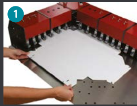
1 Place the board onto the surface and align with the top left corner plate
