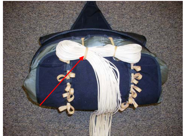
Stow another bight of the lines in the other inner stow band.
