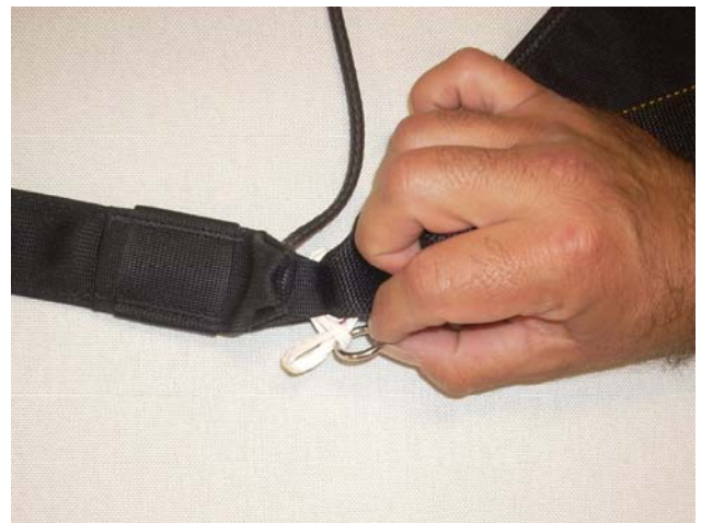
Open the Soft Link completely.
