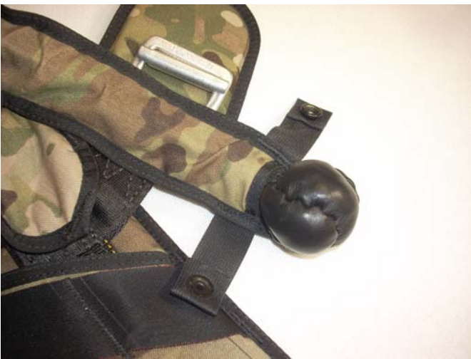
Replacement of the Connector Loop complete.
