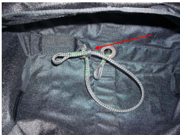
Pass the Tail Loop through the end Loop.
