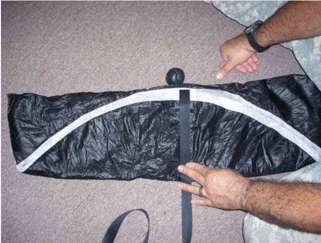
Fold the Pilot-chute into 3rds as shown.
