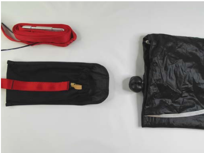
Fold the Pilot Chute in half then into 3rds as shown.
