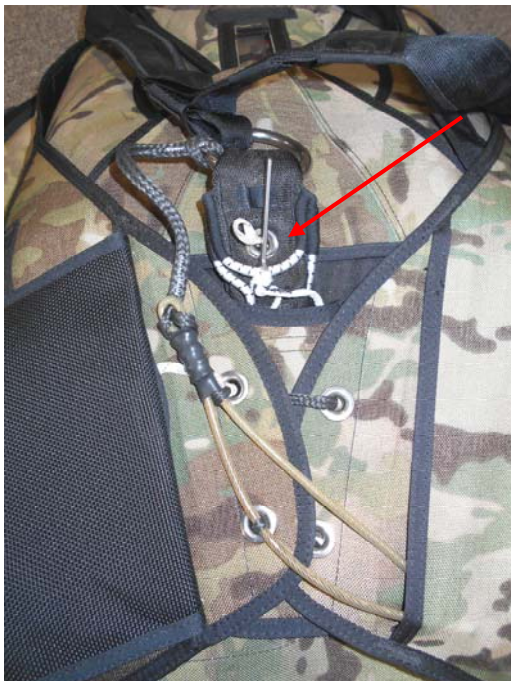
Pass the T-IIA loop through only the smallest ring then through the grommet.
