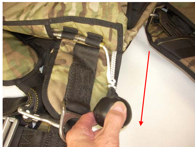
Pull the Left-Side Hacky Handle out to reveal the Connector Loop and knot.
