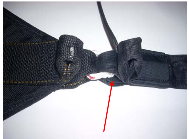
Tuck the metal ring of the Soft Link under the Bridle Loop.
