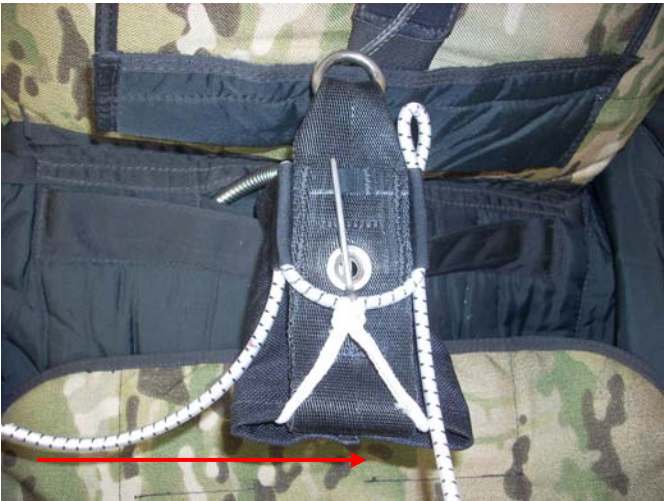
Pass the elastic through the T-8 Riser.
