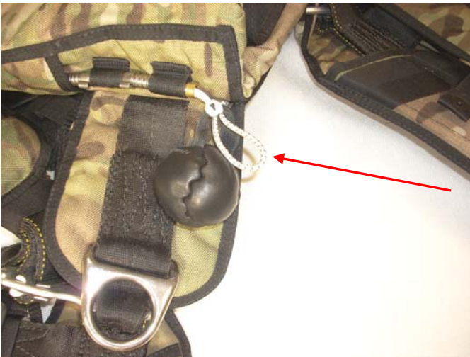
Retractable Connector Loop freed from the Left Release Hacky.
