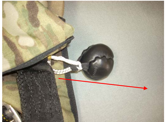
Pull the Hacky out away from the Secondary Drogue Release Housing.
