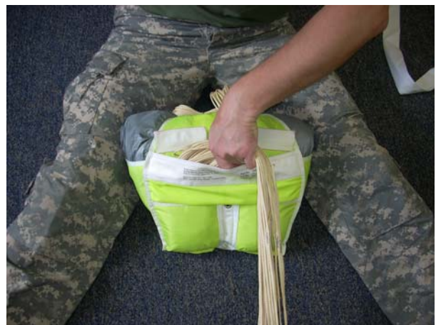
Make the first line bight and place into the corner of the line pouch.
