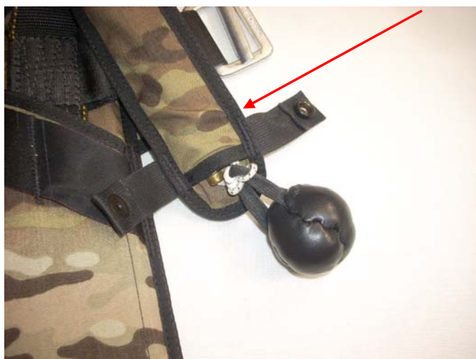
The Primary Release Handle separated from the Right Leg Pad.
