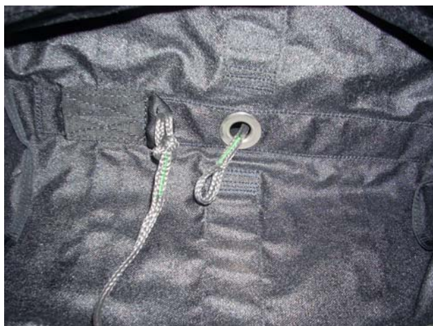
Tighten the knot formed. Bridle and Deployment Bag are now re-assembled.
