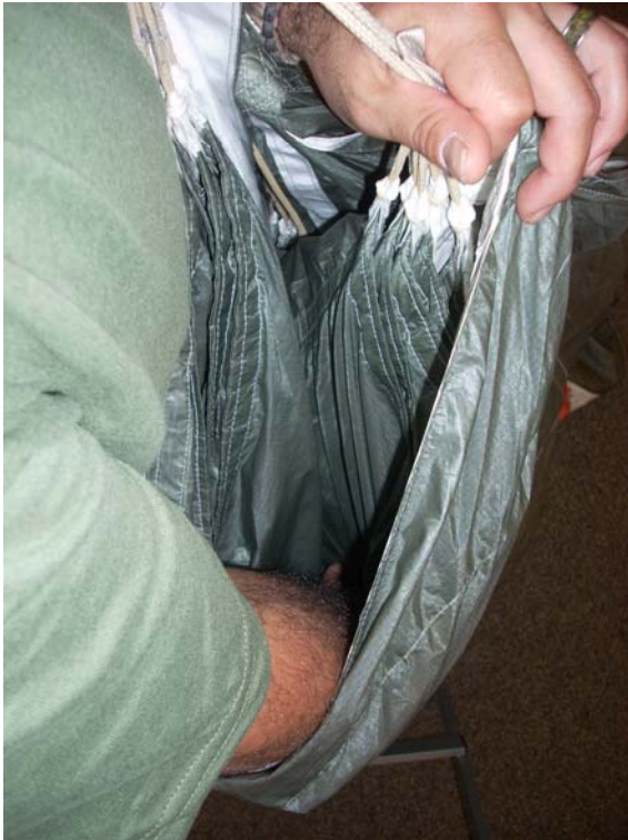
Starting with the A-line group, count the 5 right cells between the A- and B- line attachment points and flake the material away from the center of the parachute.
