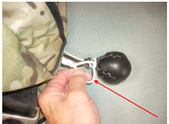
Loosen the knot of the Release Lanyard.
