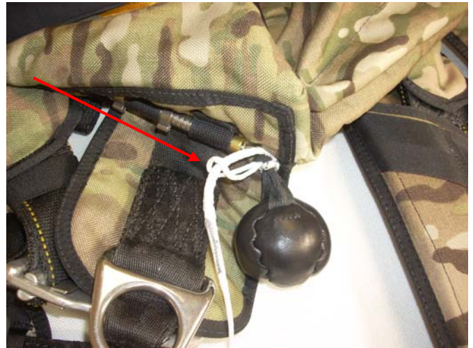
Loosen the knot of the Lanyard.
