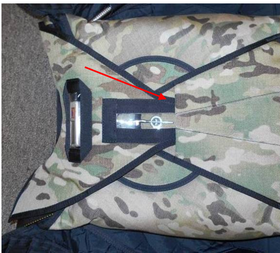
Tuck the Top Closing Flap into the slot of the Bottom Reserve Flap.
