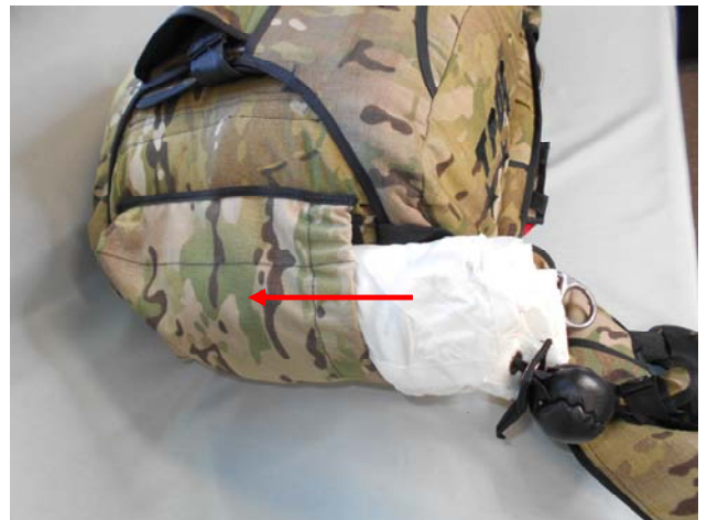
Tuck the rolled Drogue P/C into the Pouch on the bottom of the Container.
