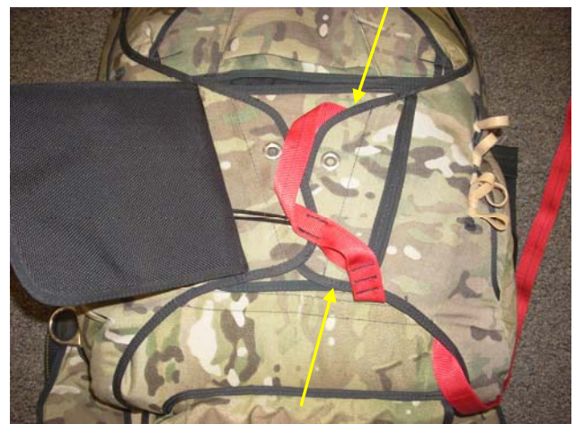
Tuck the top and bottom of the Static Line under the Right Side Flap .
