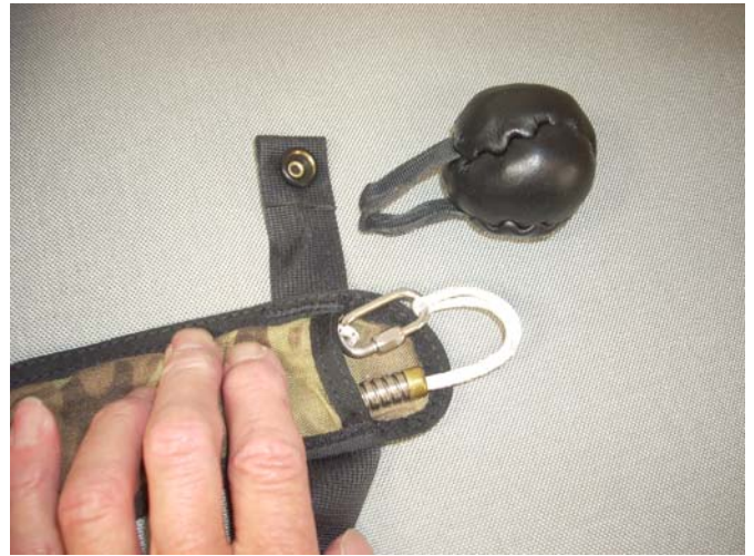
The Primary Drogue Release Hacky removed and the Elastic and Lanyard on the Rapide Link.
