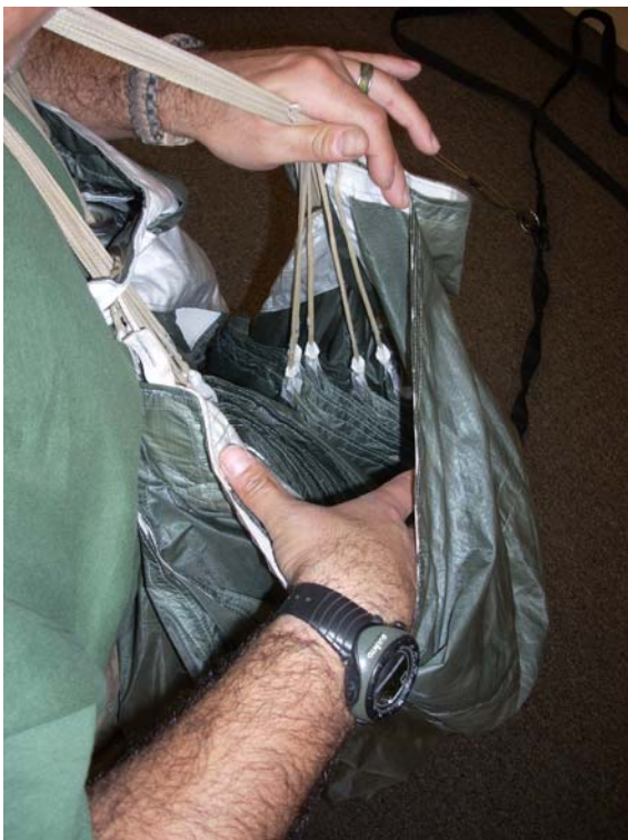
Count the 5 right cells between the B- and C- line attachment points and flake the material away from the center of the parachute.
