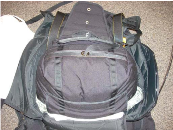
Place the Deployment Bag into the Main Container.
