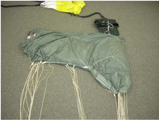
With tension on the B- and C-line groups, fold the C- line section on top of the B-lines.
