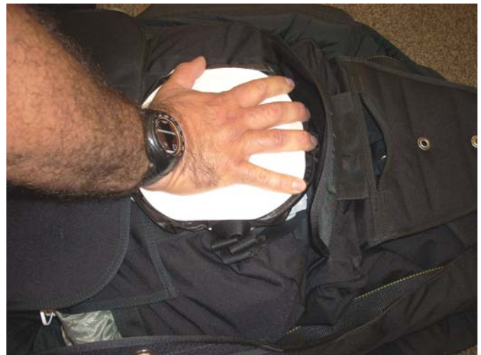
Place the Spring-loaded Pilot-chute on top of the "S"-folded Bridle and compress it keeping the canopy material folded into the spring.
