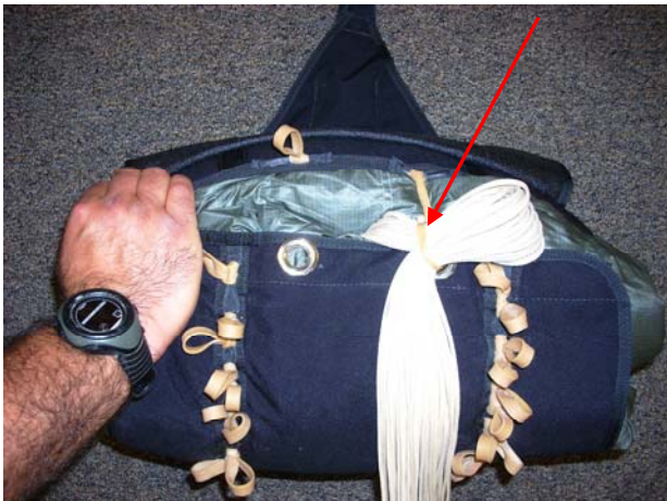
With the lines up through the center of the canopy and out of the Deployment Bag stow the lines in either of the inner stow bands of the inner closing flap.
