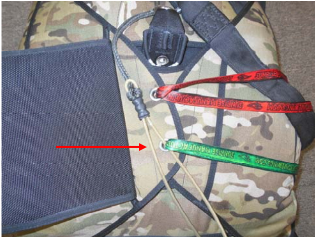
Use either of the Main Closing Pins to secure the Primary Closing Loop.
