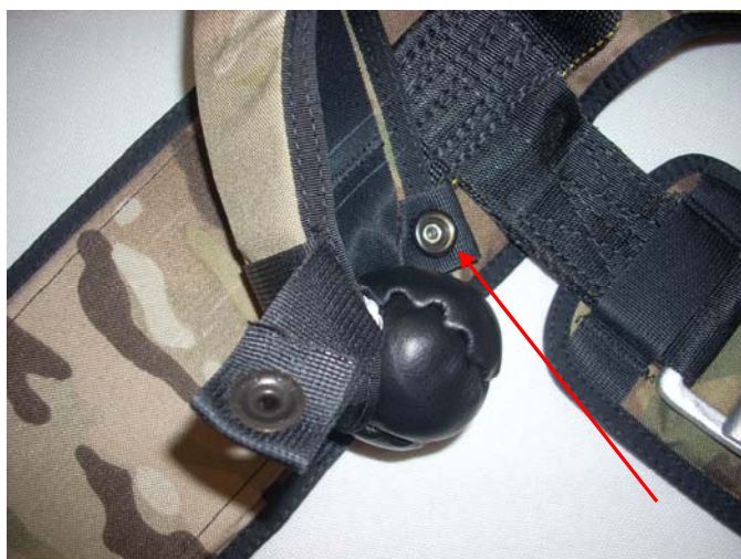
Begin to replace the Retractable Connector Loop (TPDS-HLT-309) by unsnapping the Right-Side Drogue Release Handle from the Right Leg Strap.
