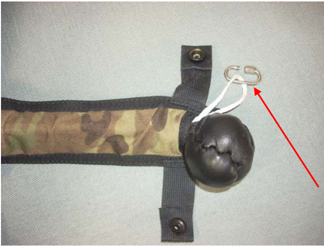
Place a Rapide Link on the Lanyard to prevent it from retracting into the housing.
