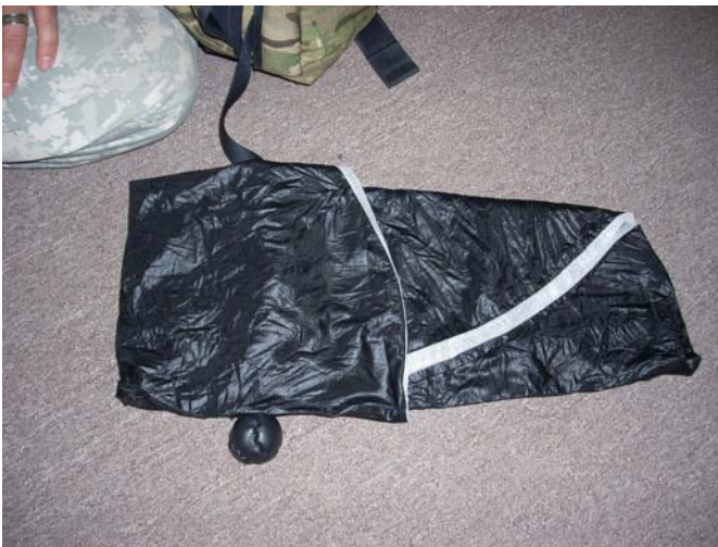
Fold the Pilot-chute into 3rd's again.
