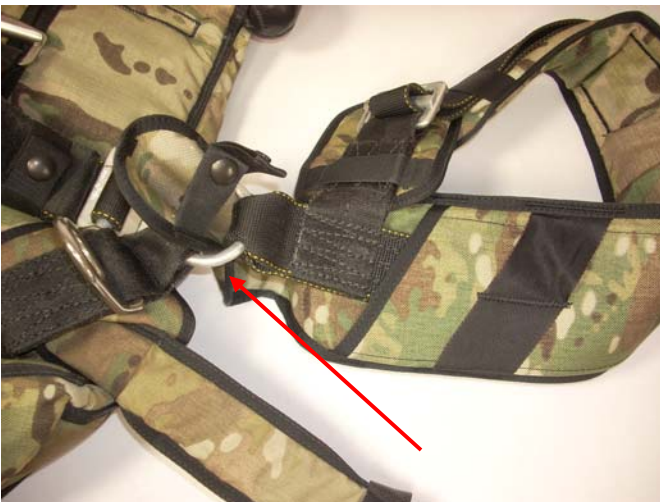
Back the Leg Pad out of the Adjustable Friction Ring. Remove Leg Strap from Friction Adapter.
