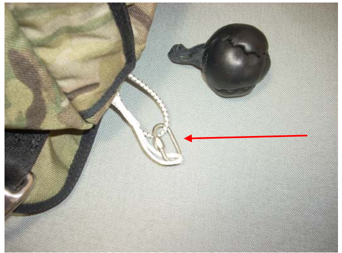
Place the Retracting Elastic onto the Rapide Link with the Release Lanyard.
