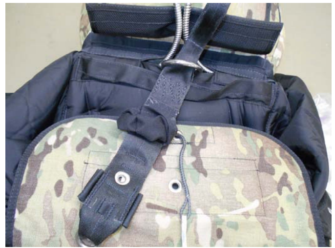
Back the Riser out of the Lark's Head knot completely and remove from the Ring.
