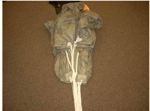
Separate the tail section, place the right control lines and material on the right side of the pack job, and the left control lines and material on the left side of the pack job.
