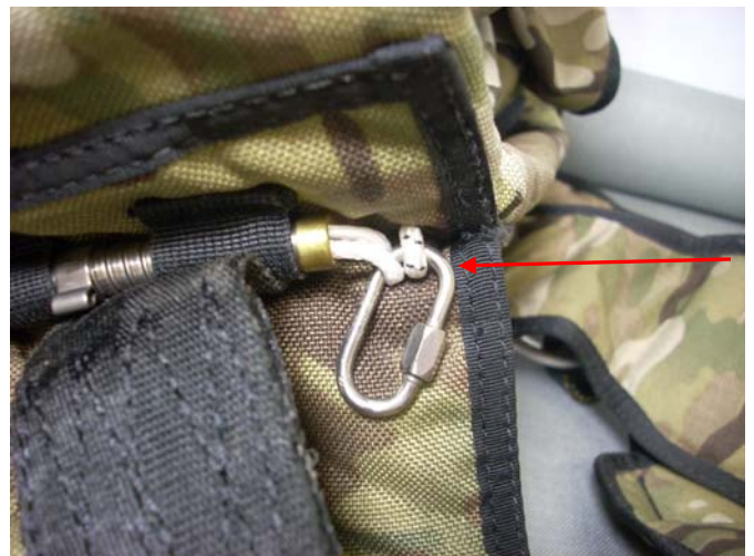
The Secondary Drogue Release Hacky removed and replaced with a Rapide Link.
