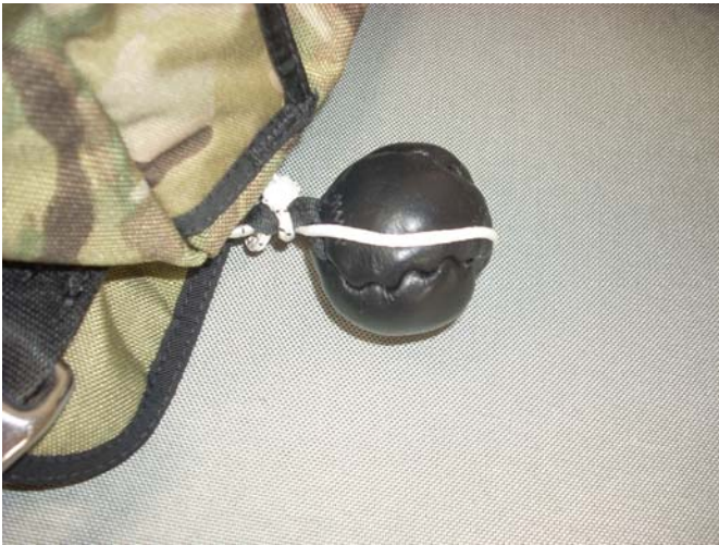
Pass the Release Lanyard loop over the Hacky.
