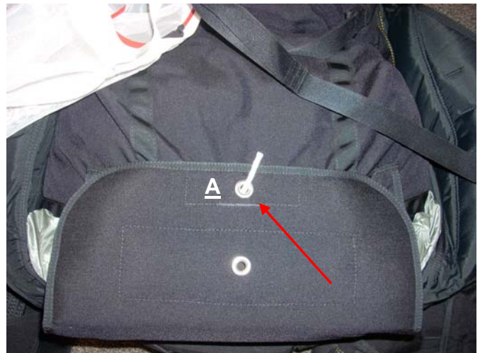
Insert a T-IIA Closing Loop into the grommet A closest to the edge of the Bottom Flap.
