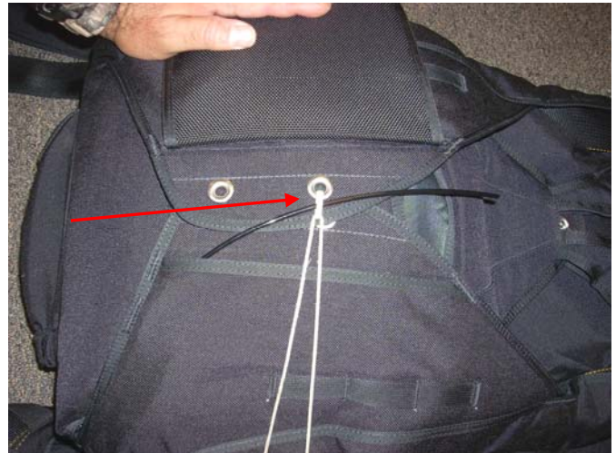
Pass the Ripcord through the Closing Loop.
