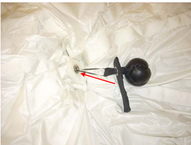
Pass the string through the grommet on the top of the Pilot Chute and pull through from the other side.
