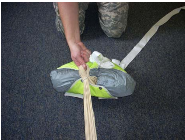
Close the Free-bag by passing the safety stow through the grommets of the Free-bag and make the first line bight approximately 1 1/2” and place in the safety stow.
