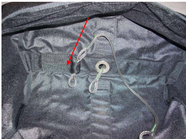
Assemble the Safety Line to the D-Bag. Begin by passing the double looped end through the T-8 loop on the bottom of the D-Bag.
