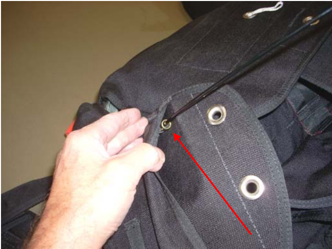
The upper end of the Ripcord Housing on the Right Closing Flap.
