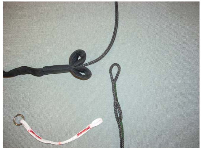
The Center Line completely removed.
