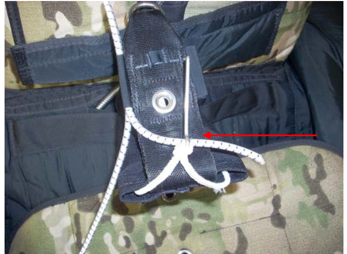
Pass the elastic through the eye of the Straight Pin. (TPDS-HLT-310)
