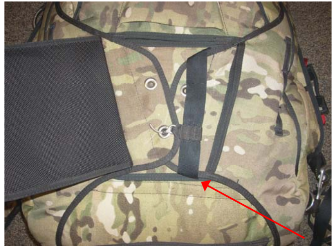
Tuck the Bridle under the Right Flap.
