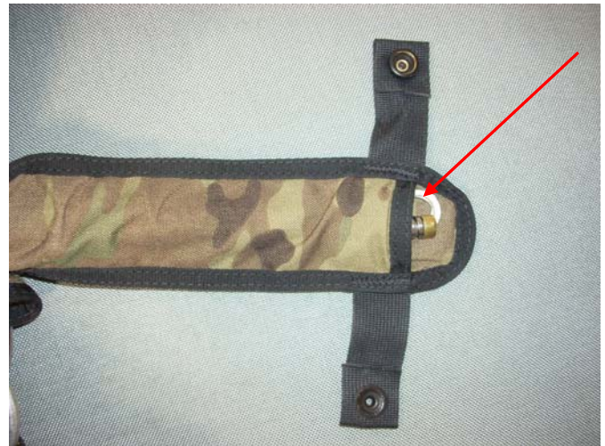
The Primary Drogue Release Hacky removed and replaced with a Rapide Link.
