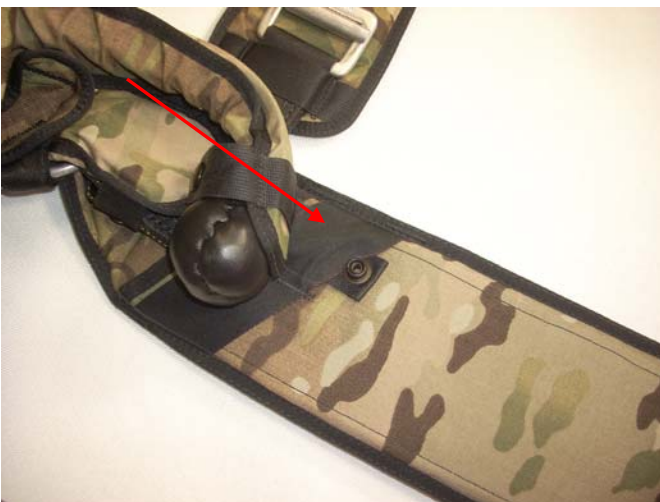
Pass the Snap Holder of the Right Drogue Release Handle under the retainer.
