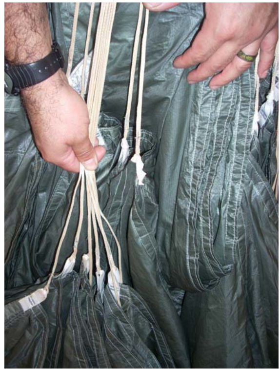
Count the 5 right cells between the D-lines and the Control Lines / tail.
