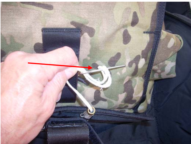
Remove the Straight Pin by loosening the knot and backing it out of the Loops of the Release Lanyards.
