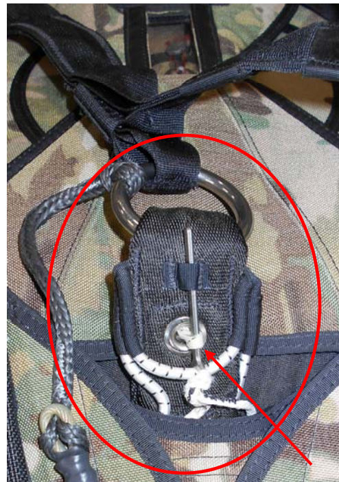
Secure the loop with the straight pin and tuck the pin end under the tape as shown.
