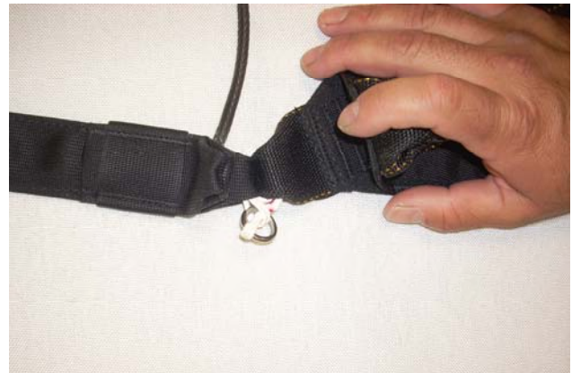
Twist the Soft Link out from the loops of the Bridle and Deployment Bag. Begin to open the Soft Link by passing the metal ring through the loop of the Soft Link.
