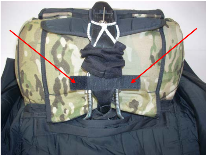
Open the Velcro Tabs that release the Housings from the 3-Ring Riser.
