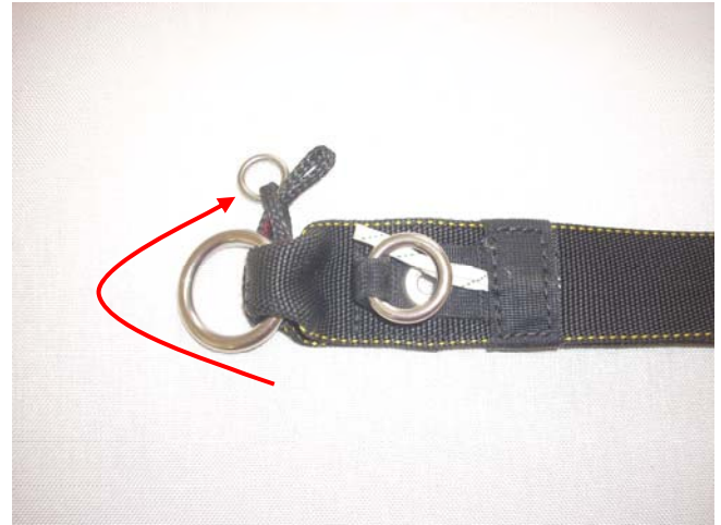
From the underside of the Riser pass the end loop through the loop beneath the mini ring.
