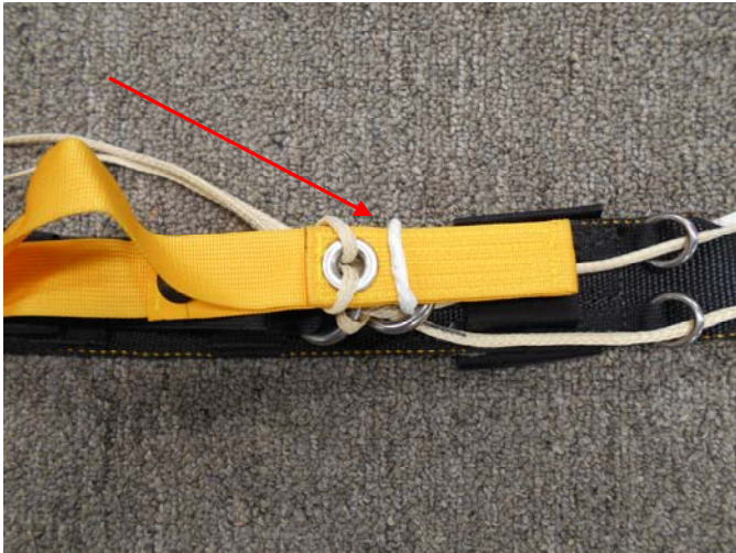
Pass the Toggle tip through the Spectra locking loop.
