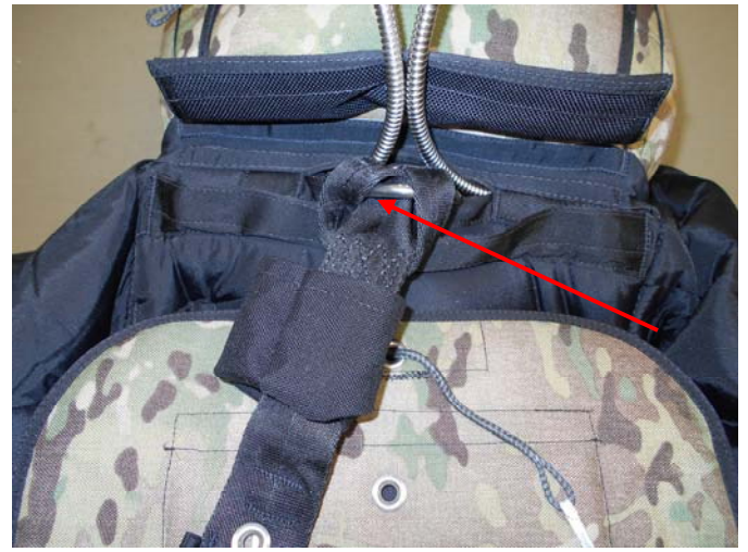
Loosen the Lark's Head knot at the ring.
