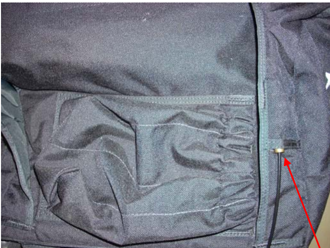
The lower end of the Ripcord Housing opening near the Drogue Pilot-chute Pouch.
