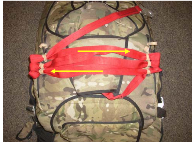
Stow the second bight of Static-line on the Left Side. Alternate back and forth leaving about 1 1/2" -2" in each bight.
