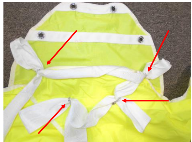
Set the Free-bag up as shown. Pull the Bridle through the Safety Stows leaving about 2 1/2” - 3” each.
