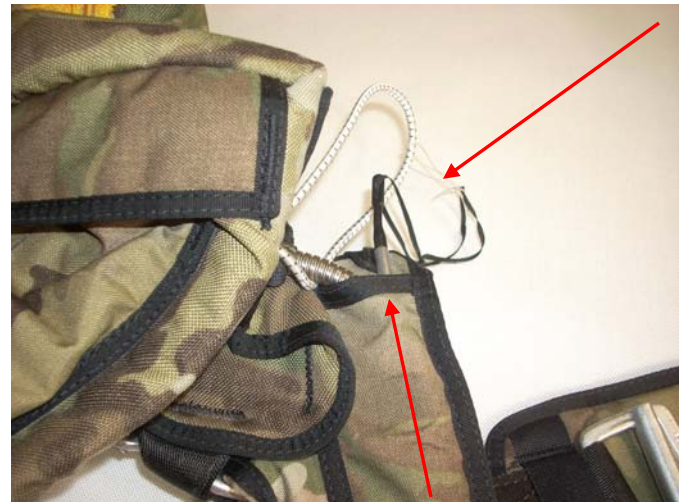
Pass the cleaning rod into the opening on the right side of the Handle Sleeve and attach the Connector Loop to it.
