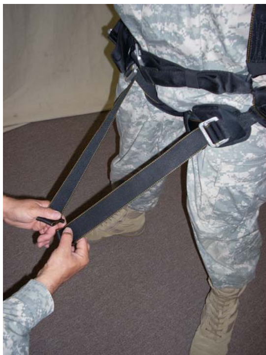
Snug the Leg Straps, making sure that the excess strap is even.
