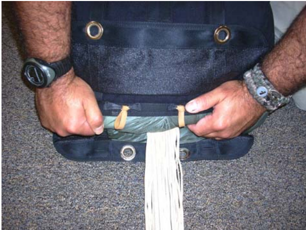
Carefully place the parachute into the Deployment Bag.
