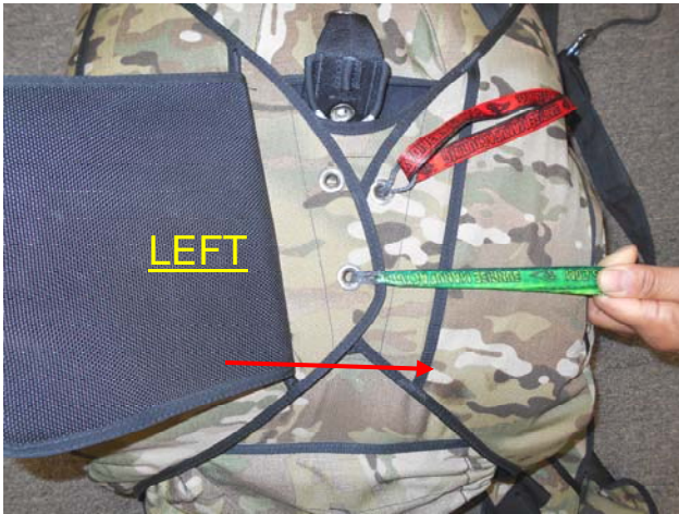
Close the Left Side Flap using the lower grommet and the Primary Closing Loop.
