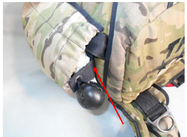
Mate the Magnet under the Pouch.
