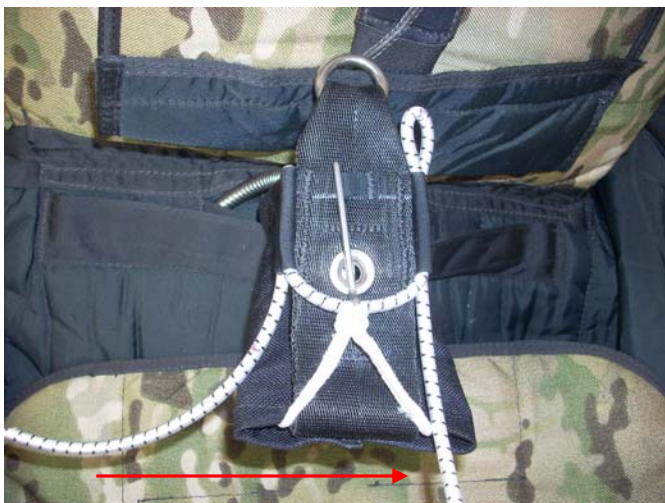
Pass the elastic through the T-8 Riser.
