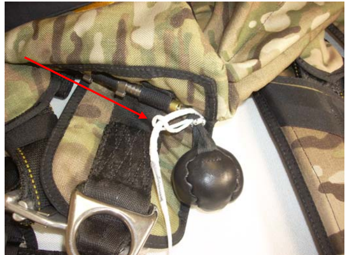
Loosen the knot of the Lanyard.
