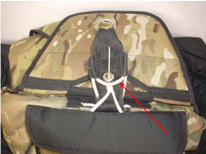
Pictured above is the Drogue Release Pin Elastic (TPDS-HLT-311) on the T-8 Drogue Release Riser.
