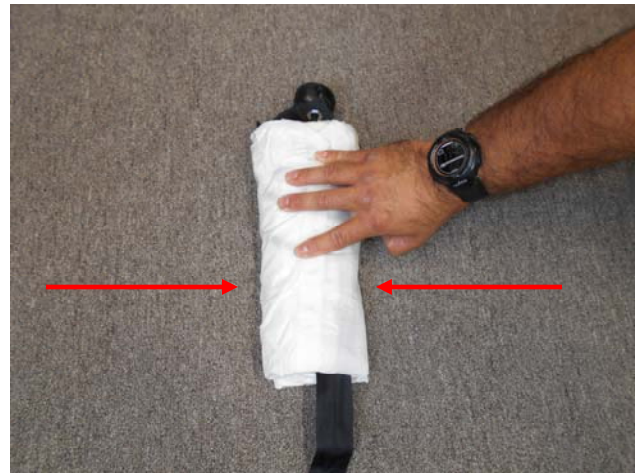
Roll both sides into the center the width of the Drogue Pouch.
