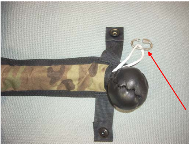
Place a Rapide Link on the Lanyard to prevent it from retracting into the housing.
