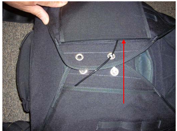
Tuck the Ripcord under the Left Flap.
