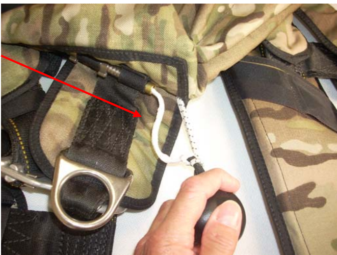
From the Left-Side Release Handle pull the Release Lanyard out of the housing.
