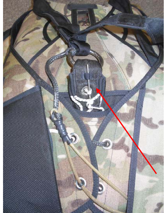
Secure the loop with the straight pin and tuck the pin end under the tape as shown.
