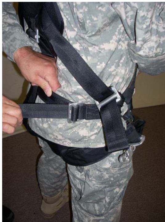
Take the slack out of the Back Strap. Make sure that it sits above the buttocks.
