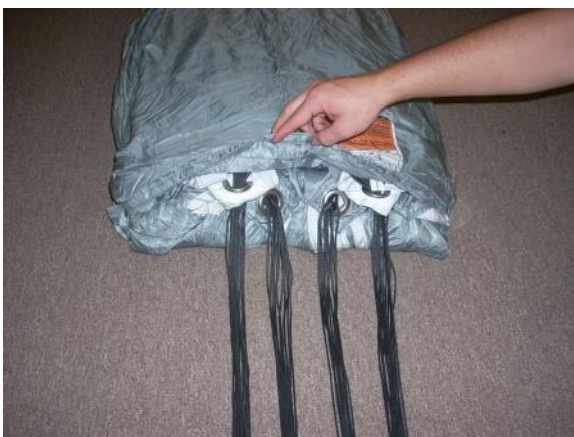
“S”-fold lower portion of canopy up to the trailing edge of the parachute and place under the trailing edge. If Needed.
