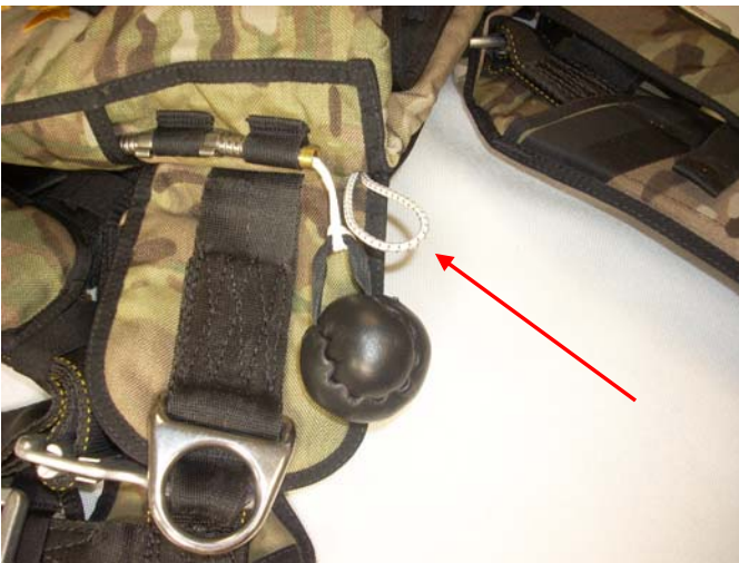
Remove completely from Hacky Handle.
