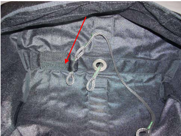
Assemble the Safety Line to the D-Bag.
