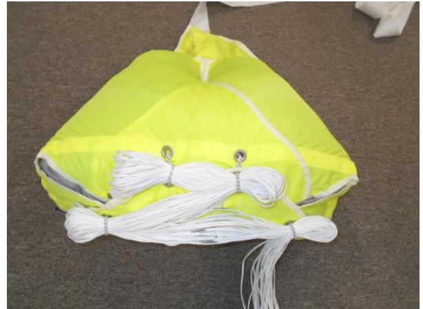
Repeat the other side. The Free-bag is ready to stow the remainder of the lines.
