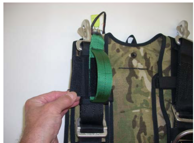
Close the Velcro covering of the Handle Pocket over the Instructor/Examiner Handle.
