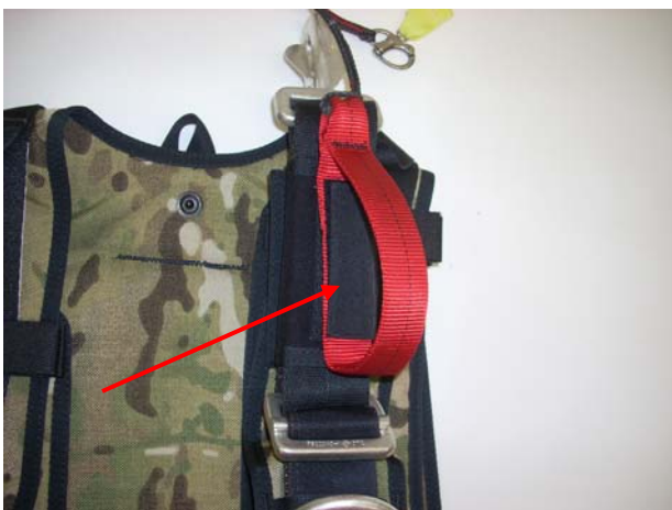
Close the Velcro covering of the Handle Pocket over the Instructor/Examiner Handle.
