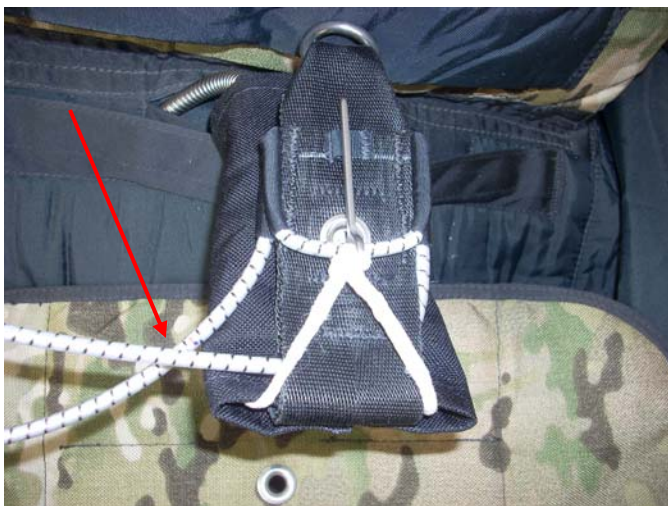
With the knots untied remove the metal clasp.
