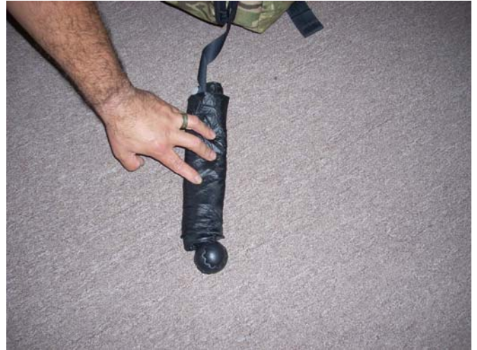
Roll the Pilot-chute towards the center.
