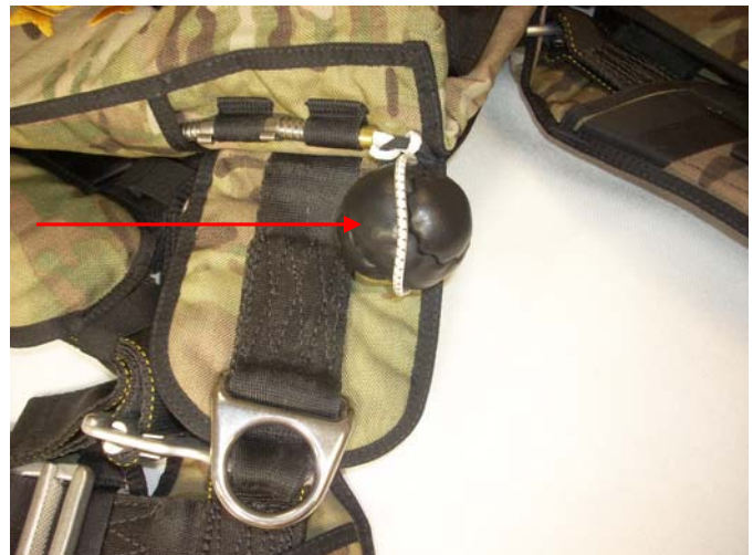
Pass the Hacky through the Connector Loop.
