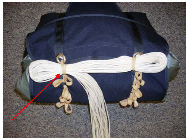
Finish closing the Deployment Bag with a bight in the last stow band.
