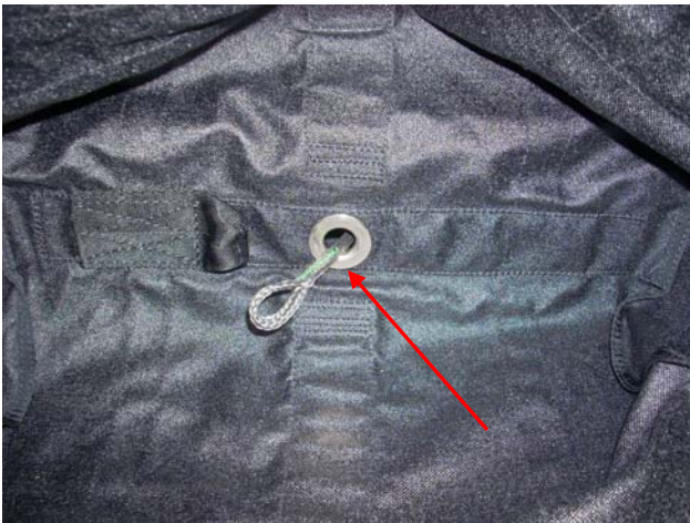
Reach between the Anti-Twist Flaps to pass the Kill-Line through the Grommet of the Deployment Bag .
