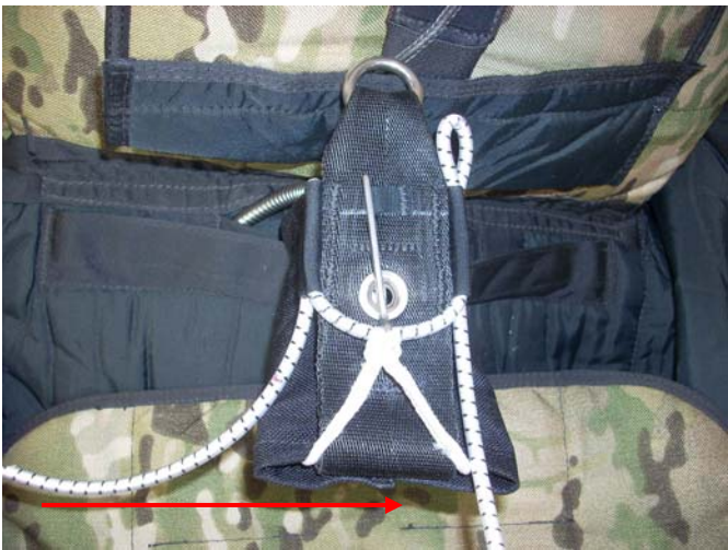
Pass the elastic through the T-8 Riser.
