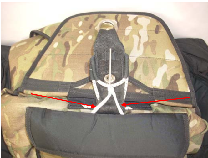
Pictured above is the 3-Ring Drogue Release Riser with the Left and Right Release Lanyards.
