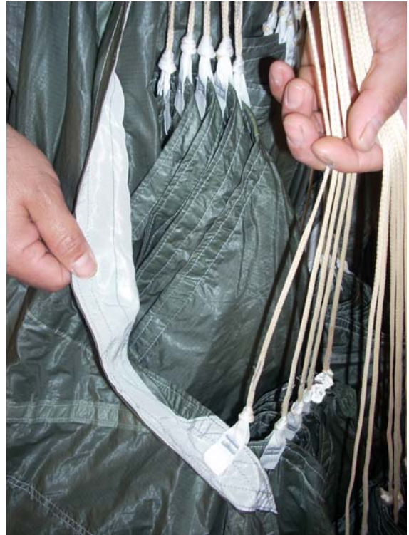
Count the 5 right cells between the C- and D- line attachment points and flake the material away from the center of the parachute.
