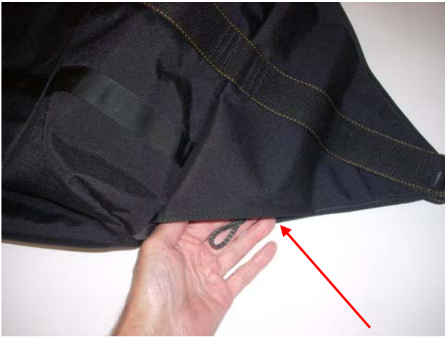
Reach between the Anti-Twist Flaps to pass the Kill-Line through the Grommet of the Deployment Bag .
