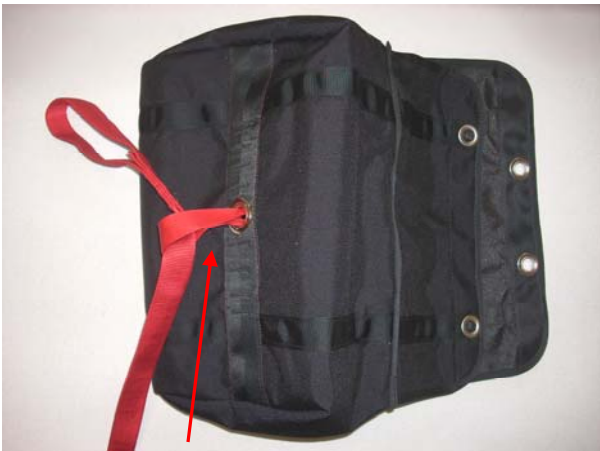
Pass the loop of the Static Line ( TPDS-HLT-264 ) through the red loop of the Main Bag.
