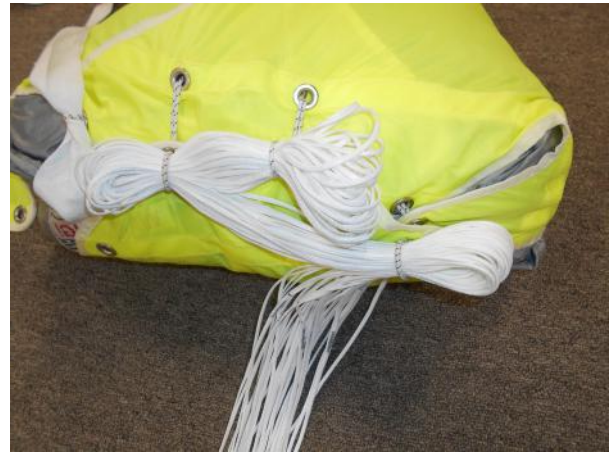
Place a line bight into the Safety Stow.
