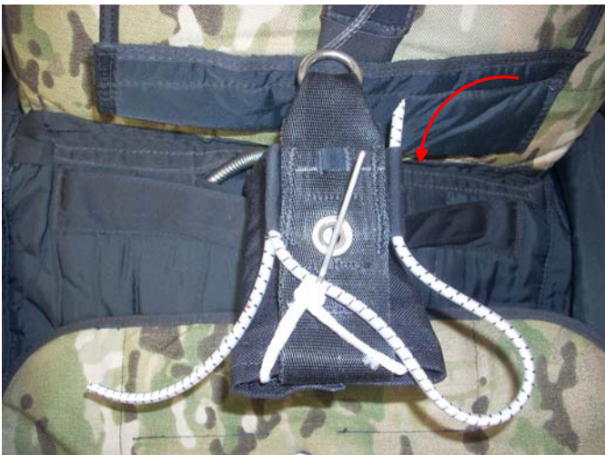
Remove the elastic from the T-3 channel.
