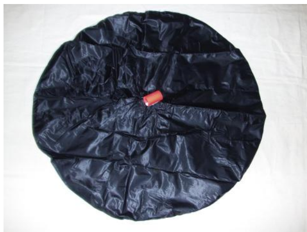
TPDS-HLT-231 Main Pilot Chute T/O Plastic Handle
