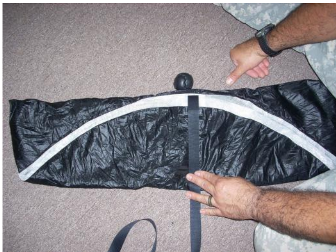
Fold the Pilot-chute into 3rds as shown.
