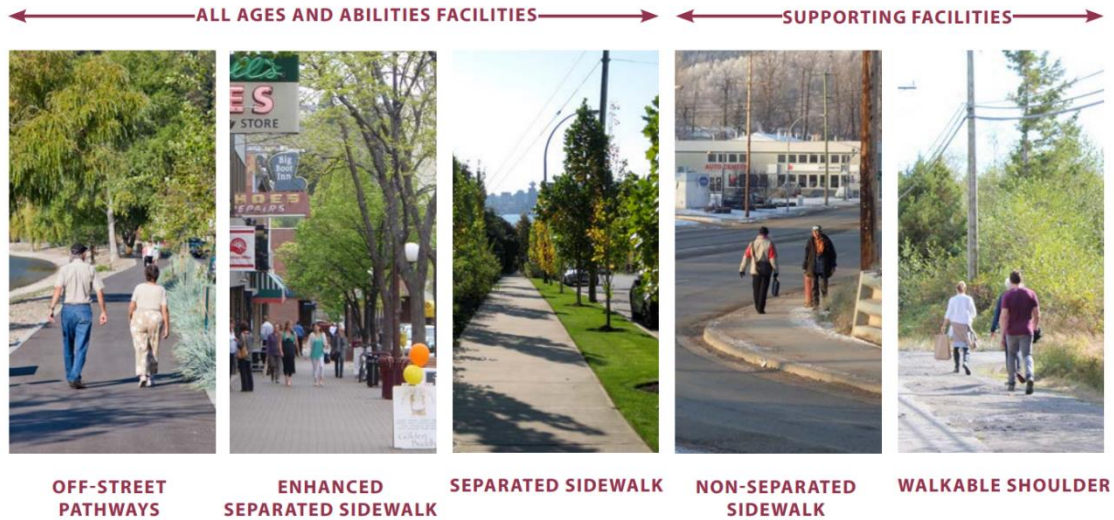
Figure 4: Pedestrian Facility Types Retrieved From: BC Active Transportation Design Guide
