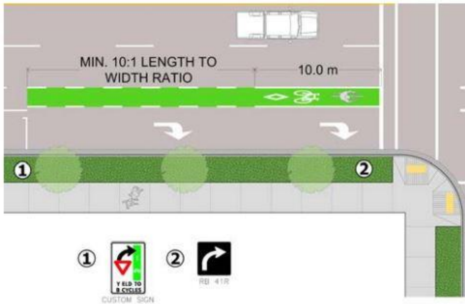
16 th Avenue and Canyon Street (top), where a person cycling is at risk of a right-hook collision from a vehicle turning right. Image on the bottom is the recommended treatment for a continuous bicycle lane with dedicated turn lane to protect cyclists on the intersection approaches. Retrieved From: BC Active Transportation Design Guide
