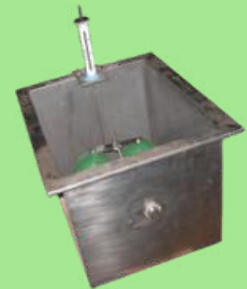
GRAVITY DOSING BOX / FOR RAPID GRAVITY FILTER PLANT
