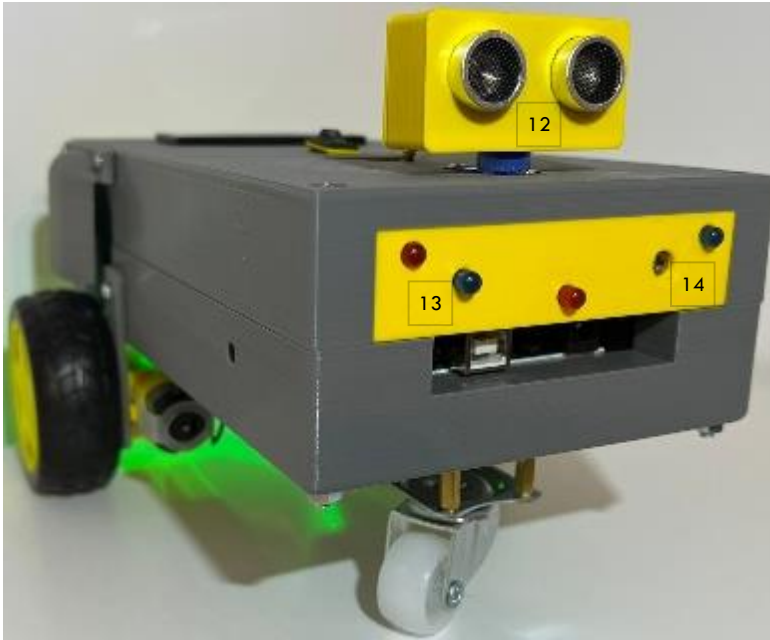
Figure 12 e) 12 - ultrasonic sensor, 13 - leds, 14 - laser diode.
