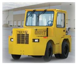
The TC-80/120 heavy duty tow tractor is a proven product with 8,000-12,000 pounds (36-54 kN) of drawbar pull.
