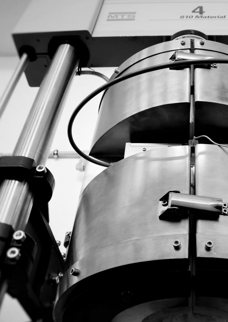
A wide variety of mechanical tests methods provided, such as: low-cycle fatigue load-controlled tests (LCF), tensile test (TENSILE), high-cycle fatigue load-controlled tests (HCF), low-cycle tatigue strain controlled tests (SCLCF), fracture mechanic tests (KIc, da / dN, combined with the possibilities of testing at a broad range of temperatures of up to 1500 ° C, makes that the Institute is at the forefront of laboratories in the world.
