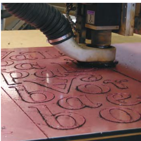
Cut Letters on Ultra Foam with Brushed Aluminum Face. Letters are nested
