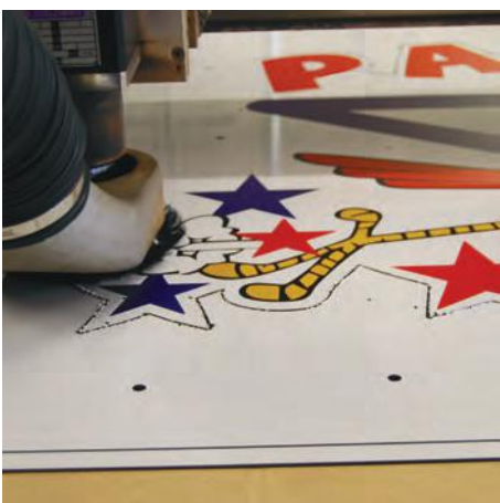
SiBond first printed on our Flatbed then cut with our Multi Cam with Icut
