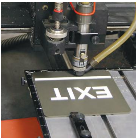
Braille Balls being applied to custom painted PVC ADA Signage
