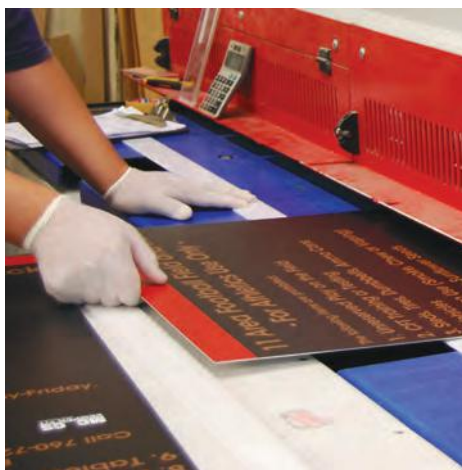
SiBond first printed on our Flatbed then cut to size with our 10' Metal Sheer
