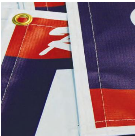
13oz banner material edges sewn for strength with grommets added
