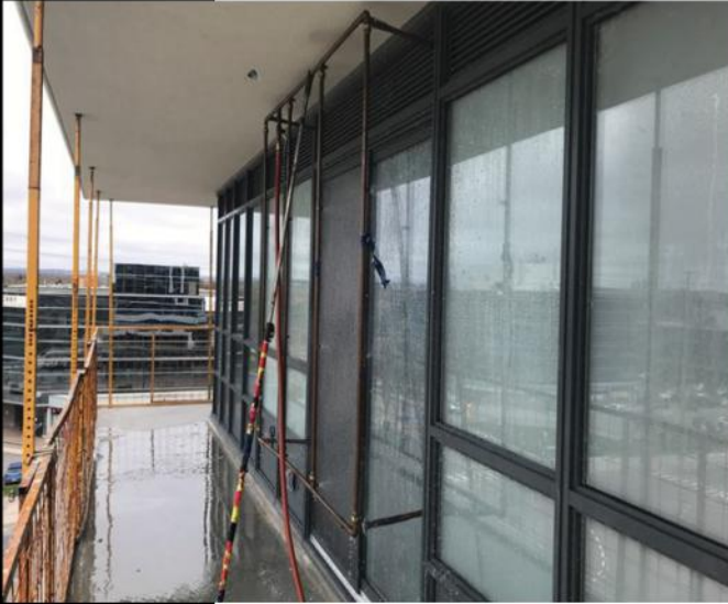
FT.01.04.A - View of spray rack on sliding doors during water penetration test.
