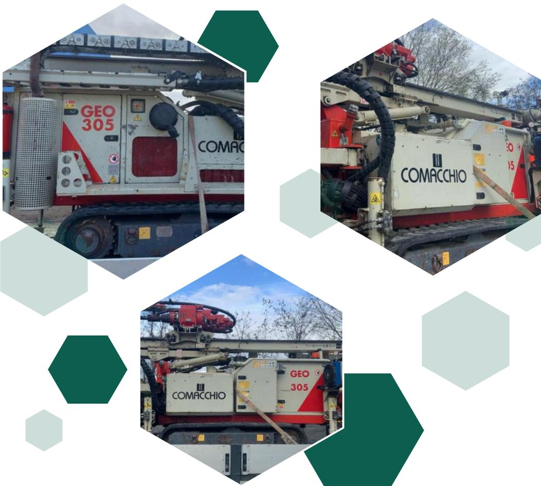
The Comacchio GEO 305 hydraulic drill rig is a powerful and reliable machine designed for geotechnical exploration and drilling in even challenging terrains. With advanced technology and sturdy construction, the GEO 305 delivers high performance, precision, and ease of use across a wide range of applications. Ideal for geotechnical engineers, geologists, and industry professionals, this drill rig is the perfect choice for efficient and safe drilling projects.
