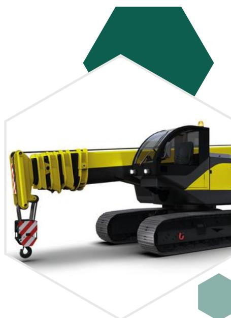
The TK40 is a compact and easy-to-maneuver crawler crane. Steering with a steering wheel, a transmission system managed by a Danfoss control unit, and its reduced dimensions allow the operator to maneuver the crane in confined areas. The crawler undercarriage with expandable track width and a height of only 3120mm ensure ease of loading and transportation. The TK40 can lift loads of up to 40 tonnes.
