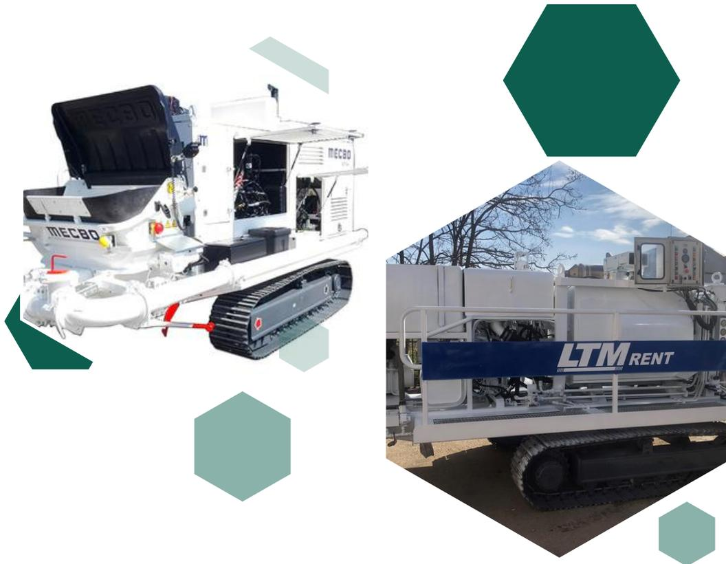
Pump installed on axle with crawler undercarriage, available with pumping unit capable of delivering up to 110 m<sup>3</sup>/h and 100 bar at the outlet and soundproof (or not) diesel engine or 132 kW/180 HP required electric motor.
