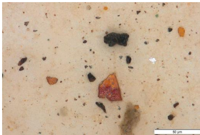
Fig 4 : (Varnish and abrasive wear – micropatch analysis)
