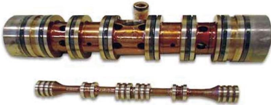
Fig 5 : Varnish deposits on spools (the primary reason for control equipment failures)
