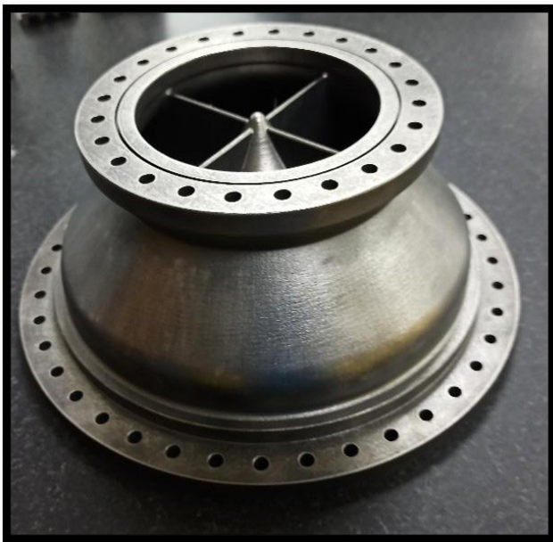
Exhaust Casing is part of C20 Engine. ISRO has conducted hot testing on this part
