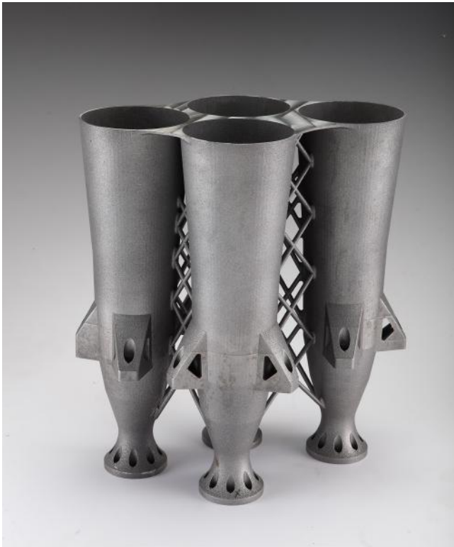
Feed Cluster is part of GSAT-19 Satellite launched on 5th June 2017. This was the first 3d Printed part from India to reach space. This is a part of Communication Satellite
