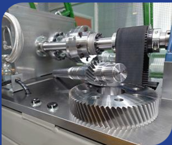
Dontyne designs and builds back-to-back test rigs for durability testing to validate changes in material, lubrication, or non involute profile
